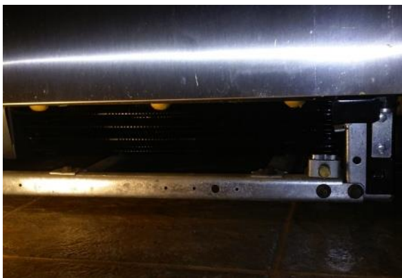
The image above (bonus point if you identified it) is a dust and lint caked coil on the bottom of a late model refrigerator. The image below is after cleaning.
